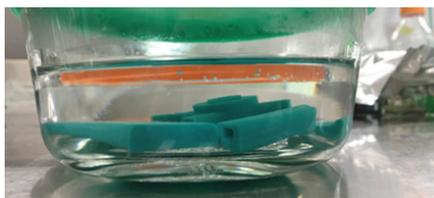
**Soak test.** Material submerged in disinfectant chemistry for 4 days with a wet/dry cycle each day. Provides data on durability of material after intense exposure to chemical.
