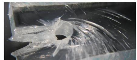
**Stress test.** Hole drilled near material edge, and vertical cut made to create high-stress area. Material immersed in disinfectant for up to 72 hours. Provides data on durability of material after intense exposure to chemical.
